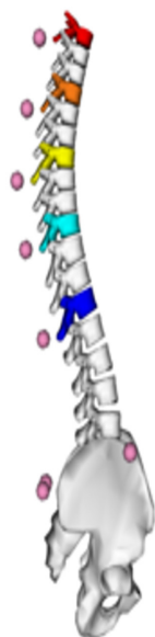
Fig. 4. Articulated kinematic model of the thoracic and lumbar spine. The thoracic vertebrae were modelled separately to increase the degrees of freedom.
