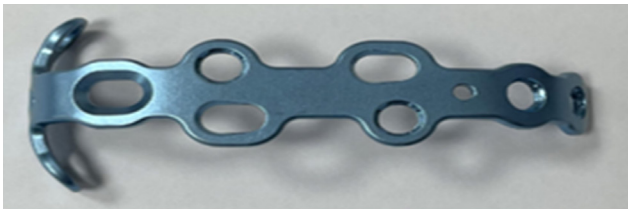
Fig. 2. Anatomically precontoured patellar plate fabricated from ASTM F67 titanium (model code 25-ANPA-209). Two 2.8-mm cortical screws can be inserted from the inferior to the superior fragment. Three 2.5-mm cortical screws and four 2.5-mm locking screws can be inserted from the anterior aspect of the plate.
