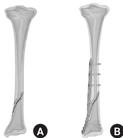
Fig. 1. The reconstructed tibial model with (A) a simulated spiral fracture and (B) an implanted medial distal locking plate.
