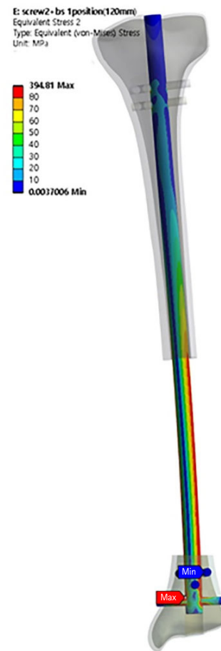
Fig. 10. The finite element method demonstrates the elastic energy of an intramedullary nail under the tension of blocking screws.
